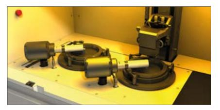
Fig. 2 View of the CeraFab Multi 2M30's flexible modular assembly
